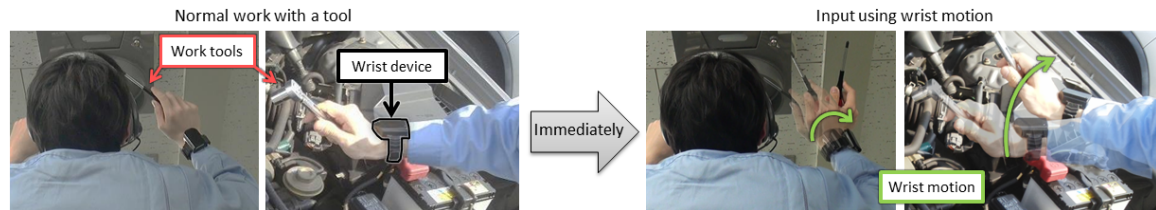
Fig. 1. An immediately-available input method that enables workers to interact with support services while performing their hand work with a tool.
